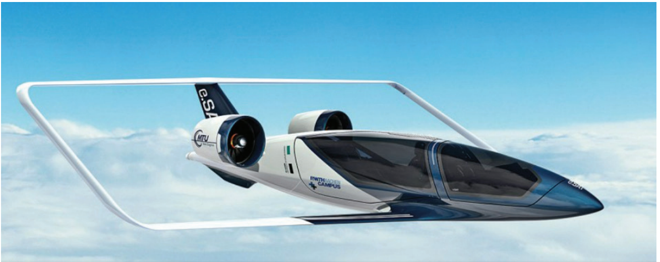
Figure 4. Artist's view of the Silent Air Taxi concept. The propulsion is ensured by ducted fans powered by a hybrid-electric powertrain. (image courtesy of e.SAT)
